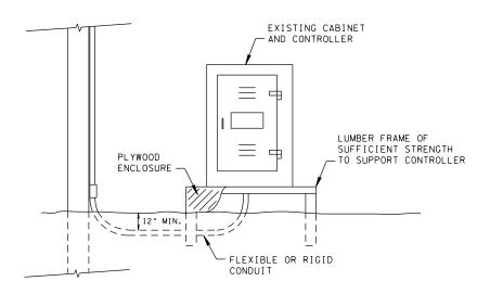
DETAIL FOR TEMPORARY RELOCATION OF EXISTING BASE-MOUNT CONTROLLER
