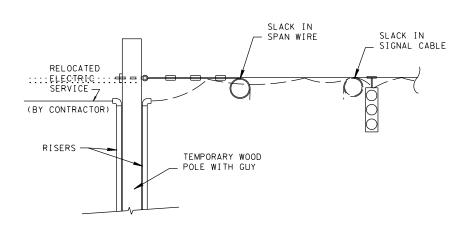
TYPICAL DETAIL FOR TEMPORARY SUPPORTS, SPANS AND CABLES (REFERENCE STANDARD DRAWING T-SG-1)
